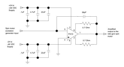
Figure 5 - Spin motor excitation signal power amplifier
