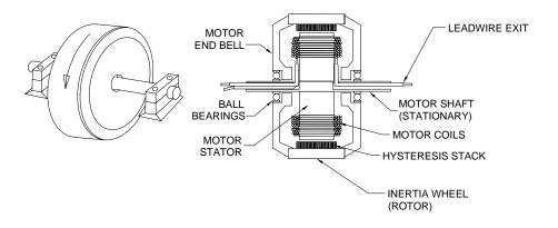
Figure 2 - Section view of hysteresis spin motor
