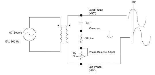
Figure 4 - Spin motor 2 phase generator
