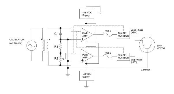
Figure 3 - Simple spin motor excitation supply block diagram
