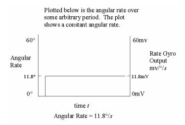
Above is a plot of *angular rate* over time. It also shows the constant angular rate. The slope of the line is 0, which is the rate of change of the angular rate. Here, there is a constant angular rate. Also the typical rate gyro output in units of millivolts (mV) per degree per second is shown on the secondary vertical axis. Here, the rate gyroscope output *scale factor* is  $1 \text{ mV}/^{\circ}/\text{sec}$ .
