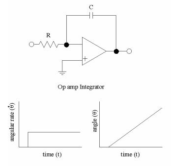
The figure above shows an op-amp integrator. The graph on the left shows an input of a constant angular rate (or the amount of rate-of-change). The graph on the right shows an output from the integrator. The sloped line represents the *integrated* (accumulating) angle turned through.
