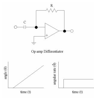
The figure above shows a basic op-amp differentiator. The graph on the left shows a constant accumulation of an angle traveled through, or of an angular rate. The graph on the right shows a differentiation of that accumulated angle, or the 'level' of the accumulating angle or angular rate.
