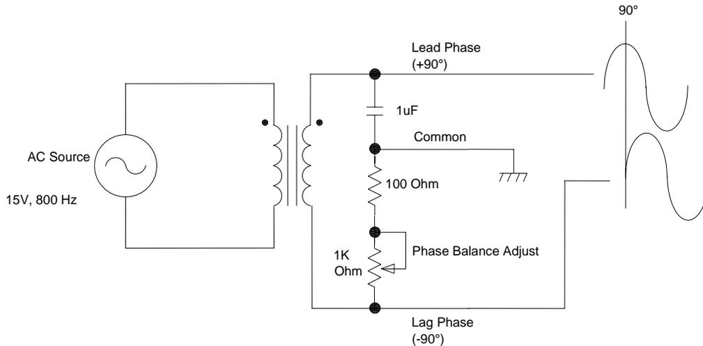
**Figure 4 - Spin motor 2 phase generator**
