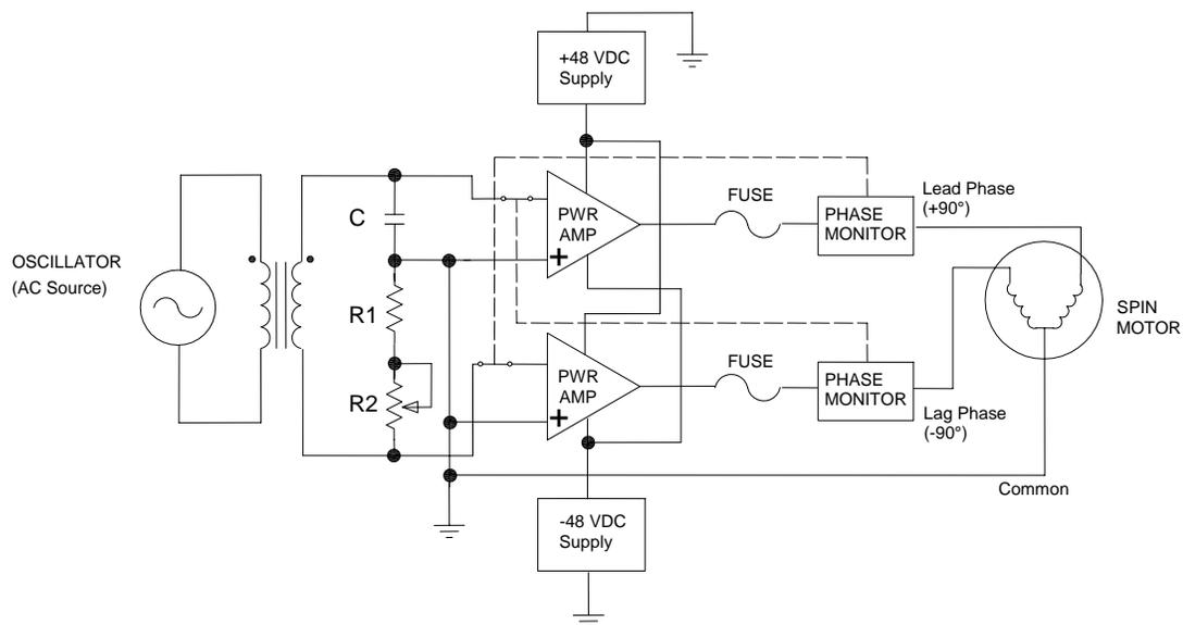
**Figure 3 - Simple spin motor excitation supply block diagram**
