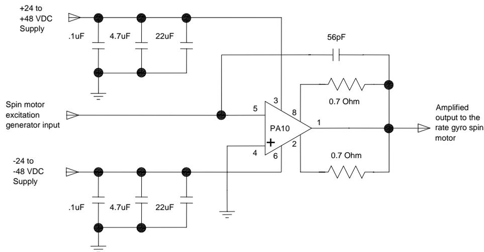
**Figure 5 - Spin motor excitation signal power amplifier**
