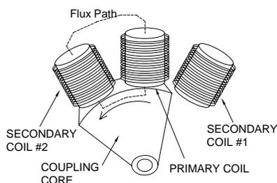
**Figure 2C - Pickoff Output – Out of Phase with Primary**
