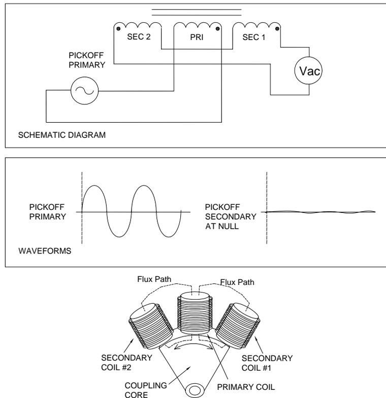
**Figure 2B – Pickoff Output – At Null**
