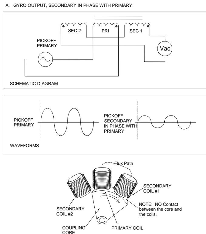
**Figure 2A - Pickoff Output - In Phase with Primary**
