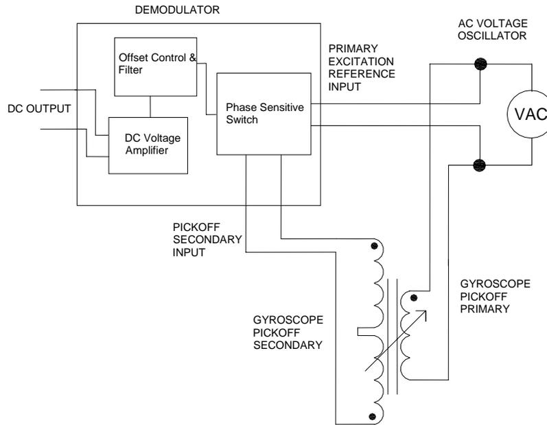
**Figure 5 – Pickoff System Block Diagram**
