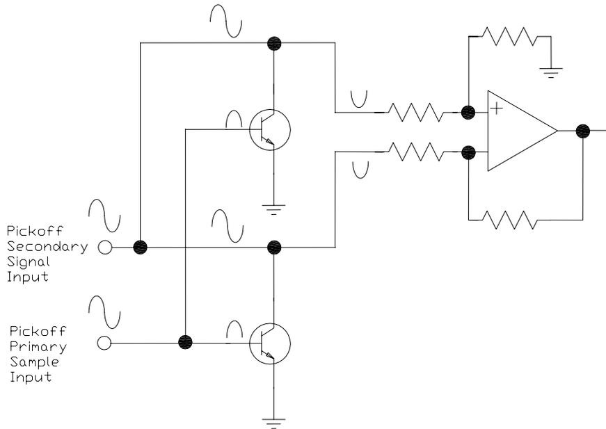
**Figure 4 – Phase Sensitive, Synchronous Rectifier**
