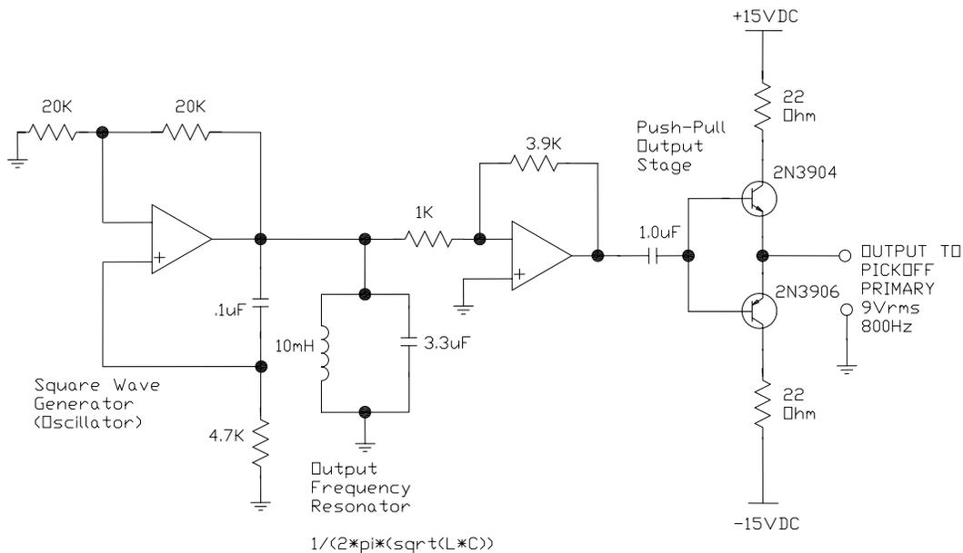
**Figure 1 – Simple AC Sinewave Oscillator**
