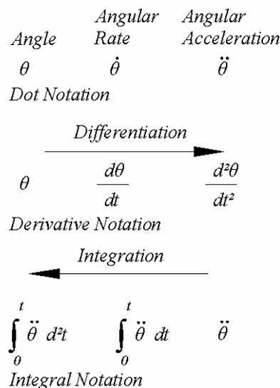
In the figure above, the operational calculus required to compute the angle traveled through, or the angular acceleration, from the rate gyroscope output is shown. If one *differentiates* the rate gyroscope output, the angular acceleration can be resolved. If one integrates the rate gyroscope output, the total accumulated angle traveled through can be resolved.
