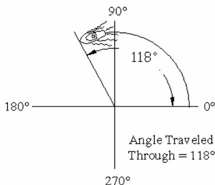
The figure above shows a ship in a  $118^\circ$  turn. The ship travels through the  $118^\circ$  arc in 10 seconds. Therefore, the ship's rate-of-turn or angular rate is  $11.8^\circ$  per second.
